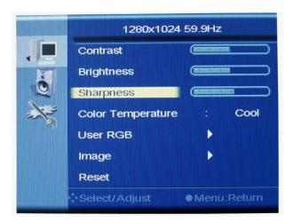
b. Press " " or " " to increase or decrease the sharpness of the display. Press "1" to confirm the adjustment and back to OSD main menu.
